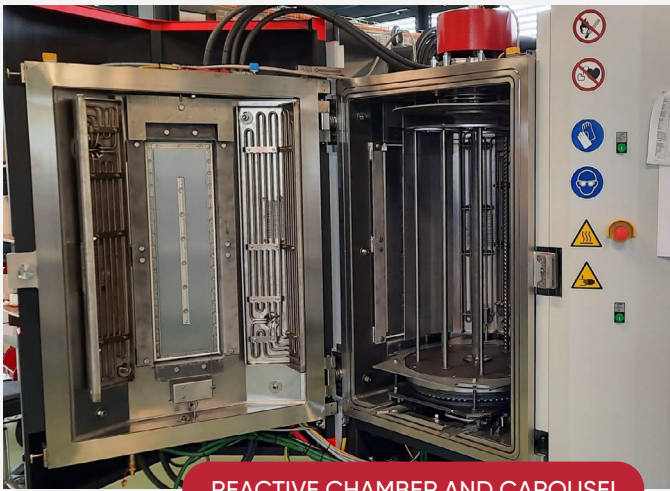
REACTIVE CHAMBER AND CAROUSEL
