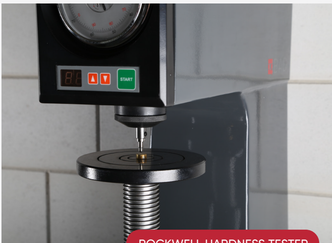
ROCKWELL HARDNESS TESTER
